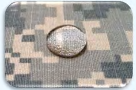
Nanotechnology-treated cloth: Becomes super-hydrophobic and the water beads up
